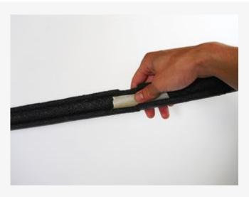
To connect two pieces of tubing together, lay a piece of tape along the middle of the tube with about half of it hanging off of the end. Pick up the second piece of track and use your finger to press the tape onto it. Use your fingers to smooth out the tape. And finally, tape the underside of the tubes together, too.
