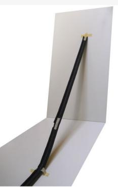
Most of the time, your students' roller coasters will need to touch down onto a flat surface like the floor. To secure the tubing to the floor, use two smaller pieces of tape and secure the sides of the roller coaster. Do not tape across the entire tube. Leaving the track clear of tape helps ensure that the marble will roll smoothly.
