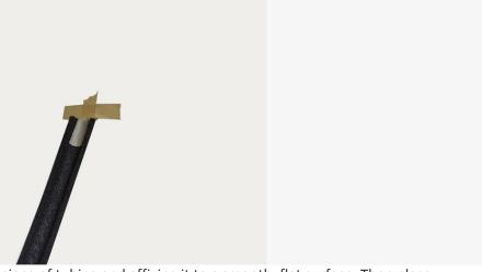
Begin by placing a strip of tape on the end of a piece of tubing and affixing it to a smooth, flat surface. Then place another piece of tape across the first piece to secure the tubing in place.
